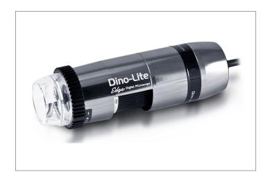
The AM7115MZT is part of the universal range and with its standard working distance and wide magnification range from 20 – 220x, it is suitable for a wide range of applications. Because of the built-in polarization filter this model is ideal when working with shiny or reflective objects such as metal, plastic, glass, jewelry, electronics, etc.
