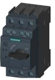
CIRCUIT-BREAKER SZ S00, FOR MOTOR PROTECTION, CLASS 10, A-RELEASE 3.5...5A, N-RELEASE 65A, SCREW CONNECTION, STANDARD SW. CAPACITY W. TRANSVERSE AUX. SWITCH 1NO+1NC
