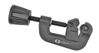
$\sim$  Adjustable pipe cutter for copper, brass, Aluminium and thin walled steel pipe  $\sim$  Easy grip handle with integral de-burring blade  $\sim$  Replaceable hardened steel cutting blade for long life performance  $\sim$  Black die cast lacquered body for strength and corrosion resistance  $\sim$  Capacity: 3-30 mm Ø Features & Benefits
