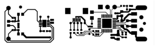
Figure 13. Si7013 Dongle Board Layout Top Layer
