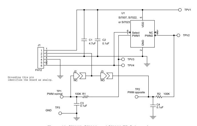
Figure 18. Si7007, Si7022, and Si7023 EB Schematic
