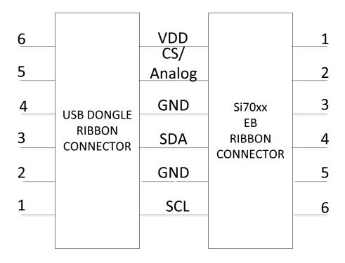
Figure 11. Ribbon Cable Pin Assignments
