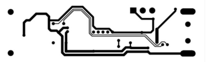
Figure 14. Si7013 Dongle Board Layout Bottom Layer
