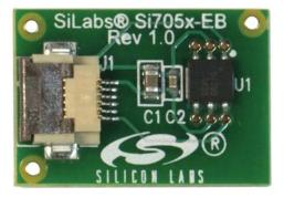
Figure 2. Si7006, Si7007, Si7013, Si7020/21, Si7022/23, and Si705x Evaluation Boards
