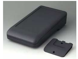
A9007218 DATEC-COMPACT L ASA+PC-FR (UL 94 V-0) lava 206x110x47mm IP 41
