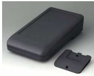
A9007208 DATEC-COMPACT L ASA+PC-FR (UL 94 V-0) lava 206x110x47mm IP 65
