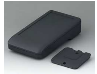
A9006218 DATEC-COMPACT M ASA+PC-FR (UL 94 V-0) lava 172x92x39mm IP 41
