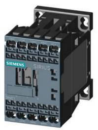
COUPLING CONTACTOR RELAY RAIL, 3NO+1NC, DC 24V, 0.7...1.25\*US, VARISTOR INTEGRATED, SZ S00, SPRING-LOADED TERMINAL
