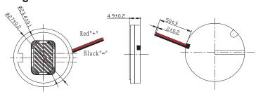
Dimensions : Millimetres Tolerance : ±0.2mm
