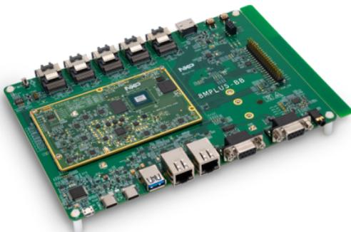
Figure 3: i.MX 8M Plus PEVK without heatsink
