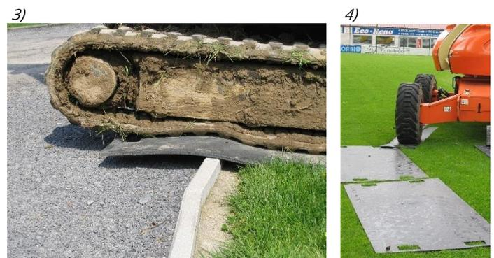
Fig. 1: Elastic deformation of a plate under heavy load
