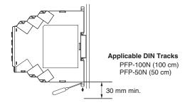
• Leave at least 30 mm of space between the product and other devices to allow easy installation and removal.
