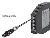
To reduce the error in the setting knob, always turn the setting knob from the minimum setting toward the maximum setting.
