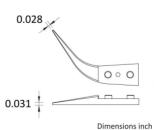
**Tip dimensions:** Tip width 0.70 mm - 0.028 inch Tip thickness 0.80 mm - 0.031 inch
