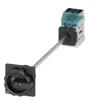
Switch disconnector 3LD3, main switch 3-polig, lu 16A operational switch at AC-23 A at 400 V 7,5 kW floor mounting Base mounting with door coupling center-hole 22,5 mm rotary operationg mechanism black  $66 \times 66$  mm
