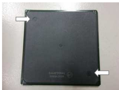
Figure 1B. Representative image of additional dimples on package top surface
