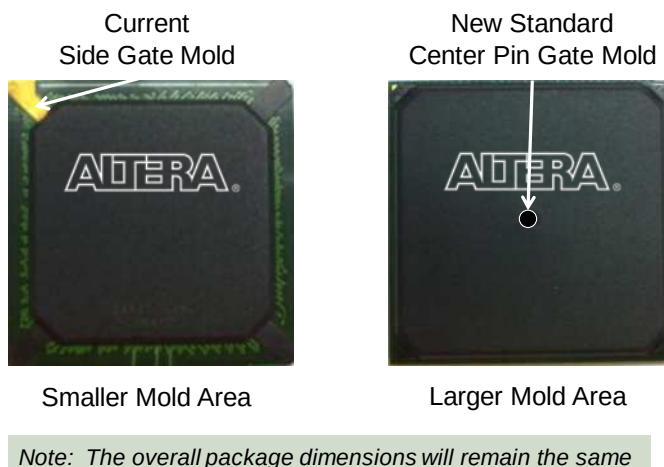
Figure 1A. Comparative images of the difference in mold compound coverage
