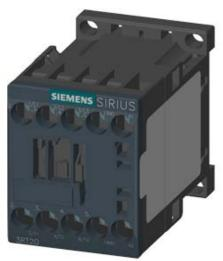
CONTACTOR, AC-3, 7.5KW/400V, 1NO, AC110V, 50/60 HZ, 3-POLE, SZ S00 SCREW TERMINAL
