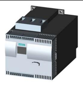
SIRIUS SOFT STARTER, VALUES WITH 460 V, 50 DEG., STANDARD: 68A, 50HP, INSIDE-DELTA CIRCUIT 3: 118A, 75HP, 200-460 V AC, 115 V AC, CAGE CLAMP TERMINALS
