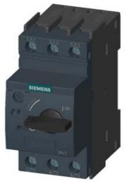
CIRCUIT-BREAKER SZ S00, FOR MOTOR PROTECTION, CLASS 10, A-REL. 0.9...1.25A, N-RELEASE16A, SCREW CONNECTION, STANDARD SW. CAPACITY
