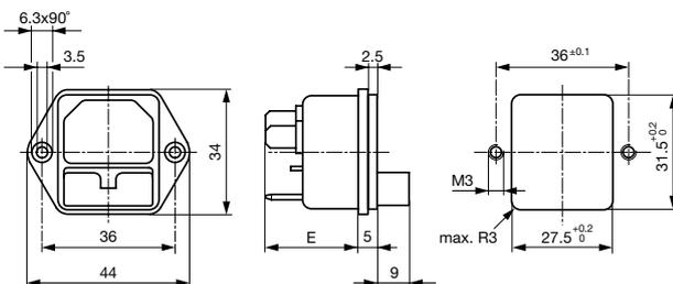
E: Lötanschlüsse 20.5 mm
