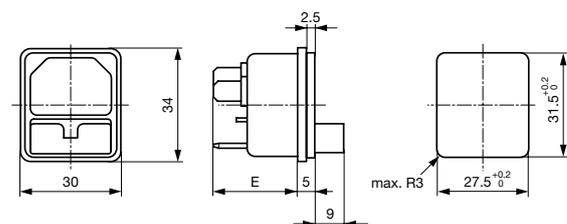
E: Lötanschlüsse 22.5 mm
