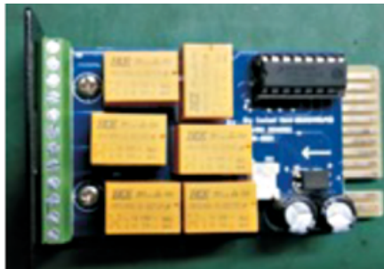
a-TroniX Relay Card for real-time monitoring of the UPS.
