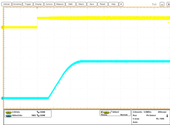
On/Off Enable Delay (Vin=5.0V, Vout=1.8V, Iout=6A, Cload=400uF) Trace1=Enable, Trace2=Vout, 2 ms/div
