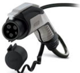
AC charging cable with Vehicle Connector, open cable end, with locking option for U-lock, with protective cap, Type 1, IEC 62196-2, SAE J1772, 32 A / 250 V (AC), Design line C-Line, Cable: 5 m, black, straight, Mating face: black, Handle area: gray
