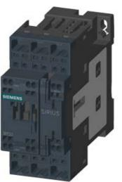
CONTACTOR, AC-3, 11KW/400V, 1NO+1NC, AC(50-60HZ)/DC ACTUAT. AC/DC 21...28V, 3-POLE, SZ S0 SPRING-LOADED TERMINAL
