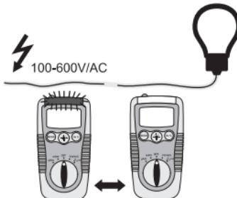
If alternating voltage is detected, the NCV display (6) lights up.
