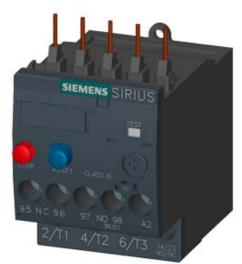
OVERLOAD RELAY 0.55...0.80 A FOR MOTOR PROTECTION SZ S00, CLASS 10, F. MOUNTING ONTO CONTACTOR MAIN CIRCUIT: SCREW TERMINAL AUX. CIRCUIT: SCREW TERMINAL MANUAL-AUTOMATIC-RESET
