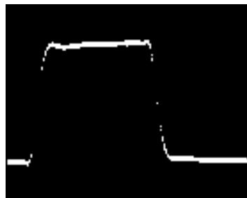
Small-Signal Transient ( A_V = -1 )
