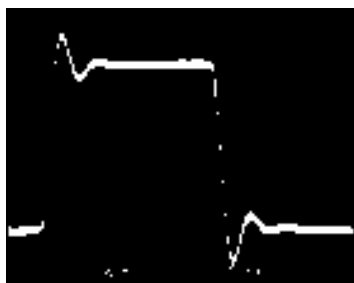
Small-Signal Transient ( A_V = 1 )
