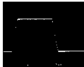
Large-Signal Transient ( A_V = 1 , C_L = 10,000\text{pF} )
