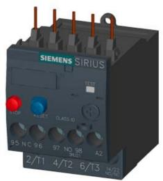
OVERLOAD RELAY 1.1...1.6 A FOR MOTOR PROTECTION SZ S00, CLASS 10, F. MOUNTING ONTO CONTACTOR MAIN CIRCUIT: SCREW TERMINAL AUX. CIRCUIT: SCREW TERMINAL MANUAL-AUTOMATIC-RESET
