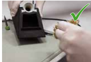
Remove dirty metal wool and empty the solder collecting box
