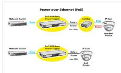
**The ROLINE Gigabit PoE Injector is a so-called PSE, a unit to supply power for e.g. surveillance cameras, and LAN devices such as access points, bridges and routers over Ethernet cable.**
