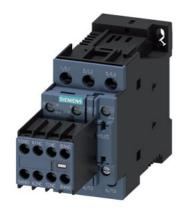
power contactor, AC-3e/AC-3, 25 A, 11 kW / 400 V, 3-pole, 24 V DC, with plugged-in diode combination, auxiliary contacts: 3 NO + 3 NC, screw terminal, size: S0, with 3RH2911-1XA22-0MA0
