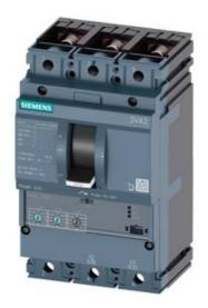
CIRCUIT BREAKER 3VA2 IEC FRAME 250 BREAKING CAPACITY CLASS L ICU=150KA @ 415 V 3POLE, LINE PROTECTION ETU320, LI, IN=250A OVERLOAD PROTECTION IR=100A ...250A SHORT CIRCUIT PROTECTION II=10 X IN BUSBAR CONNECTION
