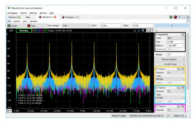
The Analog Discovery Pro (ADP3450/ADP3250) can be used with WaveForms' "Spectrum" instrument to view the power of frequency-domain components of analog signals captured on the analog input channels.
