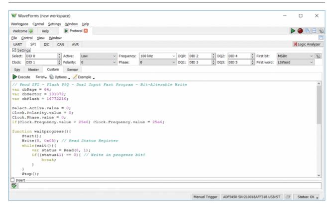
The Analog Discovery Pro (ADP3450/ADP3250) can be used with WaveForms' "Protocol" instrument to work with common communications protocols. UART, SPI, I2C, and CAN transactions can be received, transmitted, and/or spied upon by the Analog Discovery Pro
