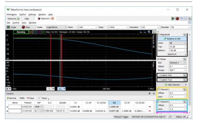
The Analog Discovery Pro (ADP3450/ADP3250) can be used with WaveForms' "Network" instrument to view the amplitude and phase response of a circuit under test. Nichols and Nyquist plots can also be viewed with this instrument.
