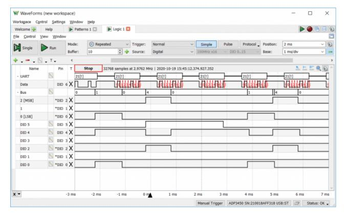
The Analog Discovery Pro (ADP3450/ADP3250) can be used with WaveForms' "Logic" instrument to act as a Logic Analyzer. When used this way, the 16 digital input/output channels are configured to capture high/low logic states on connected pins at a sample rate of up to 125 MS/s (). These channels are capable of interfacing with 3.3V and 1.2V logic signals, and when configured as inputs are tolerant of voltages of up to 5V.
