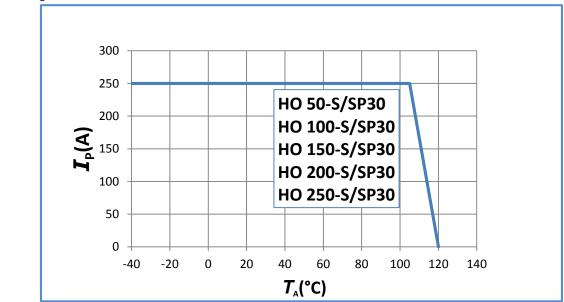
Important notice: whatever the usage and/or application, the transducer primary bar temperature shall not go above the maximum rating of 120 °C as stated in page 2 of this datasheet.
