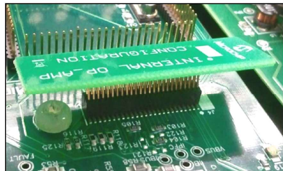
FIGURE 2: INTERNAL OP AMP CONFIGURATION BOARD
