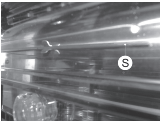
Fig. 1 The thermostat sensor "S"
