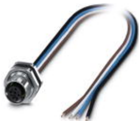
Flush-type connector, Universal, 5-position, SocketLink:M12, B-coded, Rear mounting, M16 x 1.5, Individual wires, Cable length: 0.5 m
