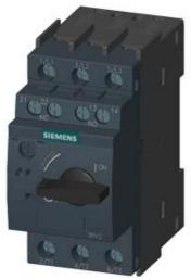
CIRCUIT-BREAKER SZ S00, FOR MOTOR PROTECTION, CLASS 10, A-REL. 2.2...3.2A, N-RELEASE42A, SCREW CONNECTION, STANDARD SW. CAPACITY W. TRANSVERSE AUX. SWITCH 1NO+1NC
