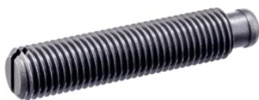
Grub screws are clamping screws that can directly transmit forces via the thrust point. The pressure surface of the thrust point of the steel version is hardened.
