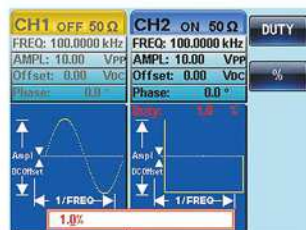
1% Duty Cycle of Square Wave
