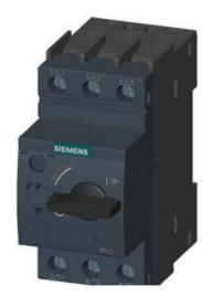
CIRCUIT-BREAKER SZ S0, FOR MOTOR PROTECTION, CLASS 10, A-REL. 9..12.5A, N-REL. 163A, SCREW CONNECTION, STANDARD SW. CAPACITY STANDARD SW. CAPACITY
