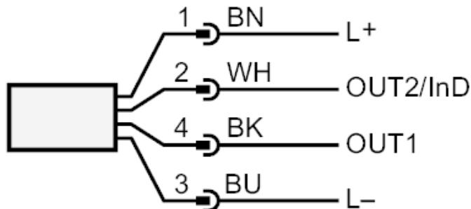
OUT1: switching output volumetric flow quantity monitoring
