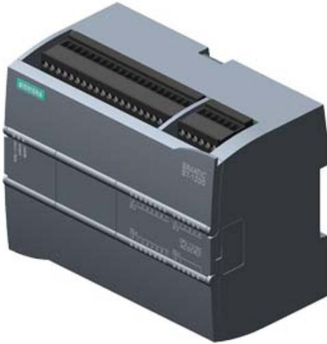
SIMATIC S7-1200, CPU 1215C, KOMPAKT CPU, AC/DC/RELAIS, 2 PROFINET PORT, ONBOARD I/O: 14 DI 24VDC; 10 DO RELAIS 2A, 2 AI 0-10V DC, 2 AO 0-20MA DC, STROMVERSORGUNG: AC 85 - 264 V AC BEI 47 -63 HZ, PROGRAMM/DATENSPEICHER 100 KB
