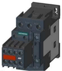
CONTACTOR, AC-3, 18.5KW/400V, 2NO+2NC AC110V 50HZ/120V 60HZ 3-POLE, SZ S0 SCREW TERMINAL PERMANENT AUX. SWITCH FOR SUVA APPLICATIONS
