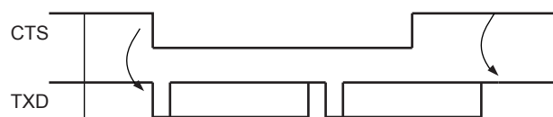
Figure 44-28: Transmitter Behavior when Operating with Hardware Handshaking
