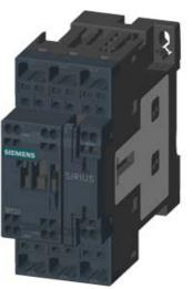
CONTACTOR, AC-3, 7.5KW/400V, 1NO+1NC, AC(50-60HZ)/DC ACTUAT. AC/DC 200...280V, 3-POLE, SZ S0 SPRING-LOADED TERMINAL
