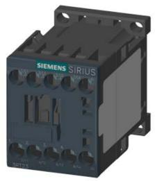
4NO CONTACTOR, AC1: 18A AC 110V 50/60HZ 4-POLE, 4NO, SZ: S00, SCREW TERMINAL
