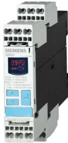
DIGITALES UEBERWACHUNGSRELAIS FUER DREIPH. SPANN. MIT N-LEIT ZUSCHALTBARE PHASENFOLGE PHASENAUSFALL 3X 160 BIS 690V AC 50 BIS 60 HZ UNTER- UND UEBERSP. 160-690V HYSTERESE 1-20V JE 0-20S FUER UMIN UND UMAX 1 W FUER UMIN 1 W FUER UMAX FEDERZUGKLEMME
