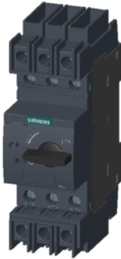
LEISTUNGSSCHALTER BGR. S0, FUER DEN ANLAGENSCHUTZ, MIT APPROBATION CIRCUIT-BREAKER UL 489, CSA C22.2 NO.5-02, A-AUSLOESER 20 A, N-AUSLOESER 260 A, SCHRAUBANSCHLUSS, STANDARDSCHALTVERMOEGEN
