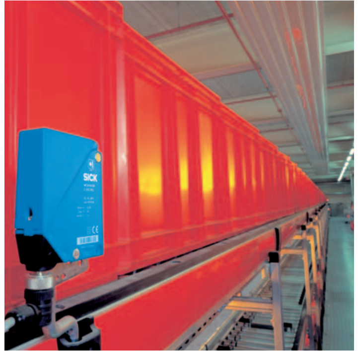
◀ The WT34 photoelectric proximity switch stands out for its large scanning distance with regard to checking whether second or backward storage bays are occupied.
