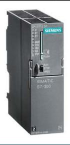
SIMATIC S7-300, CPU317-2 DP, CENTRAL PROCESSING UNIT WITH 1 MBYTE WORKING MEMORY, 1. INTERFACE MPI/DP 12MBIT/S, 2. INTERFACE DP-MASTER/SLAVE, MICRO MEMORY CARD NECESSARY
