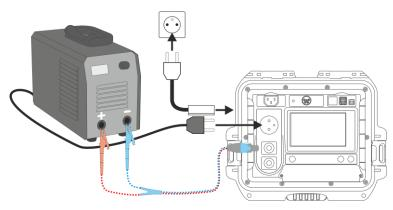
Measurement with PAT-3F-PE adapter. Connecting a 1-phase 230 V appliance.
