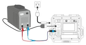
**2b** Variant with powering the welding machine directly from the mains socket.
