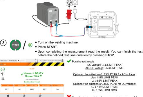
$\checkmark$  Negative test result: U<sub>0</sub> does not meet at least one of the above conditions. .
