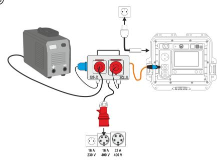
Measurement with PAT-3F-PE adapter. Connecting a 3-phase 32 A appliance.
