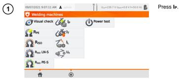
Before starting the measurement, similarly to **sec. 4.2**, following parameters must be set: **test duration, limit, polarity** and **test method**.
