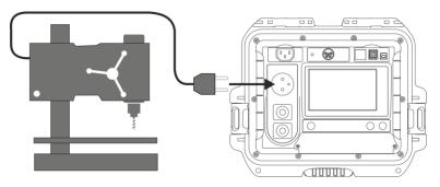
For Class II and accessible parts disconnected from PE in Class I: connect the probe to **T2** terminal socket and touch the accessible parts of the tested appliance.
