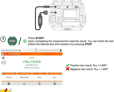
Test circuit is electrically isolated from the mains and from mains' PE lead.
