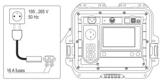
The device is powered from mains 195...265 V, 50 Hz.
