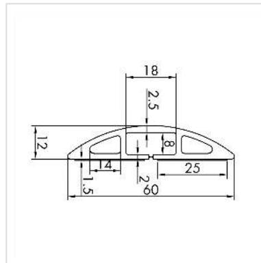
**The cable bridge not only covers the cables lying on the floor, it also prevents tripping. The cable bridge has three cable passages that separate data and power supply cables - to prevent signal interference.**
